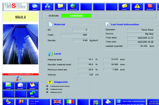
Interface for controlling silos
